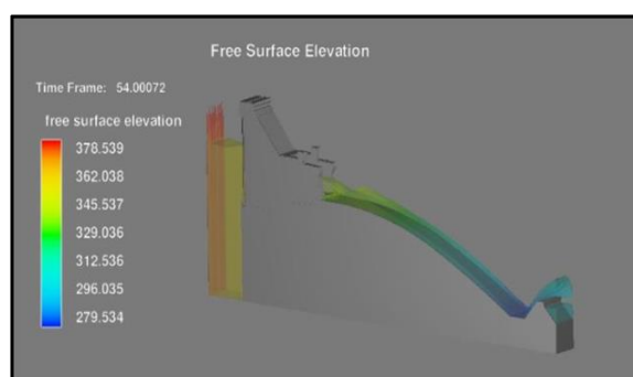
Fig. 4 Flow Simulation at 10.67 m Gate Opening
